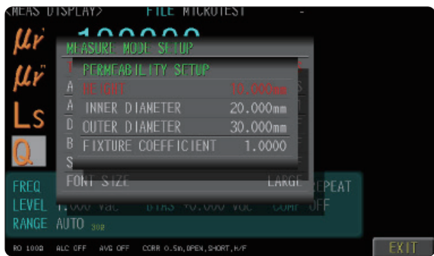
Magnetic Material Test Fixture (FX-0000C8) Using the magnetic material test fixture for measuring of permeability of various toroidal cores or ferrite cores and electromagnetic shielding coating materials. 6630 built-in formula to directly calculate the permeability coefficient value \mu' , \mu'' .
