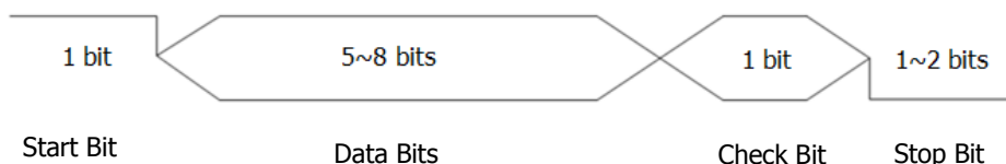
Figure 5-13 Schematic Diagram of RS232 Protocol
