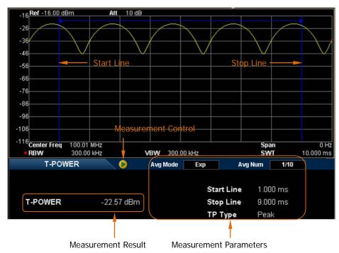
Figure 2-14 T-Power Measurement Interface
