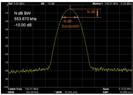
Figure 2-25 N dB BW measurement
