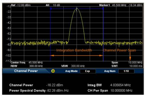
Figure 2-16 Channel Power Measurement Interface
