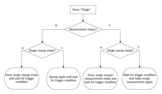
Figure 2-10 Process of Single Sweep
