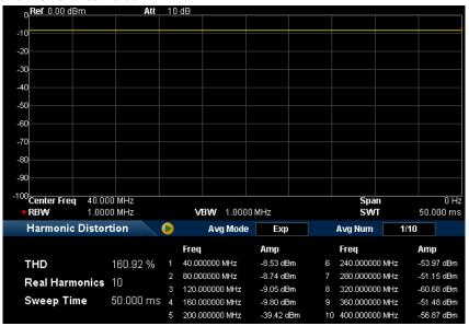
Figure 2-20 Harmonic Distortion Measurement Interface
