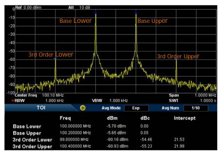
Figure 2-21 TOI Measurement Interface
