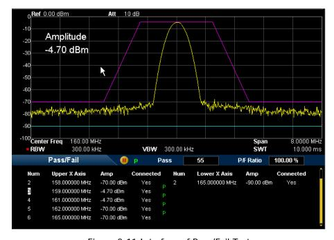
Figure 2-11 Interface of Pass/Fail Test
