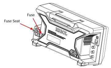
Figure 1-16 To Replace the Fuse
