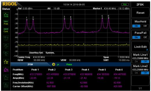
Figure 2-22 2FSK Measurement Interface
