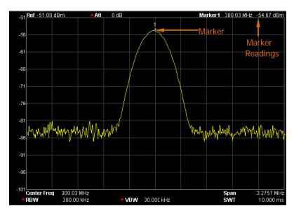
Figure 2-23 Schematic of the Marker
