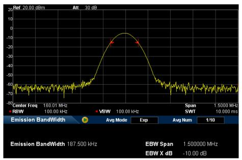
Figure 2-18 EBW Measurement Interface
