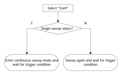
Figure 2-9 Process of Continuous Sweep
