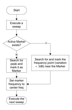
Figure 2-1 Process of Signal Track
