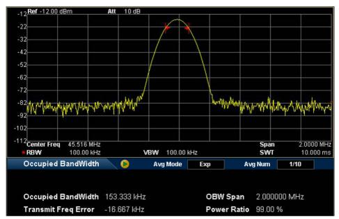
Figure 2-17 OBW Measurement Interface
