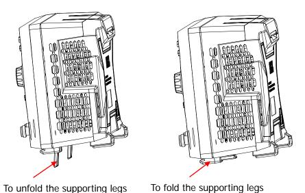
Figure 1-3 To Adjust the Supporting Legs
