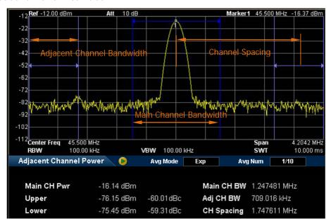
Figure 2-15 Adjacent Channel Power Measurement Interface
