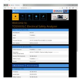
Turn ON Identify: "LXI Web Identify" appears in the front panel display of the connected TOS93. This allows you to identify the connected TOS93.
