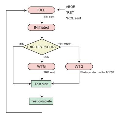
To start a test immediately, set the trigger source to IMM, and then use the INIT command.
