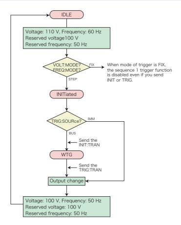
The TRIGger:TRANsient:SOURce command sets the trigger source to BUS or IMMediate.
