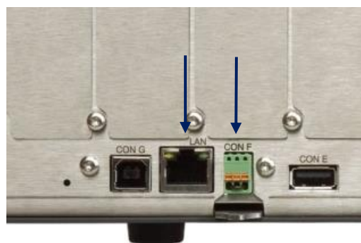
fig 5 - 6 The location of the LAN-connector (left) and the Interlock connector (right) at the rear panel.
