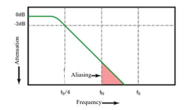
Figure 11-3 Sampling Rate and Oscilloscope Bandwidth
