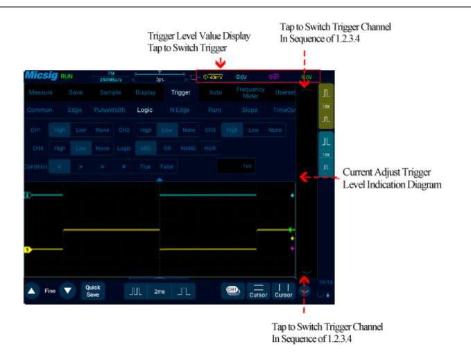
Figure 6-21 Trigger Level Adjustment
