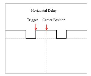
Figure 6-7 Horizontal Delay
