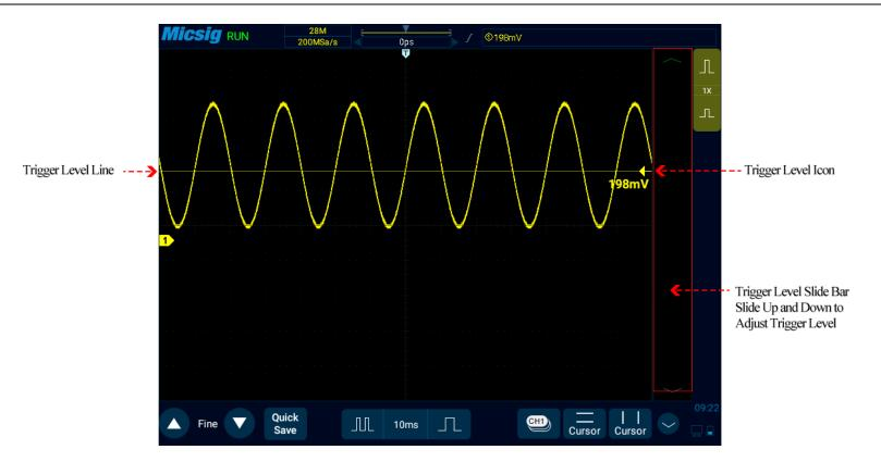
Figure 6-8 Trigger Level
