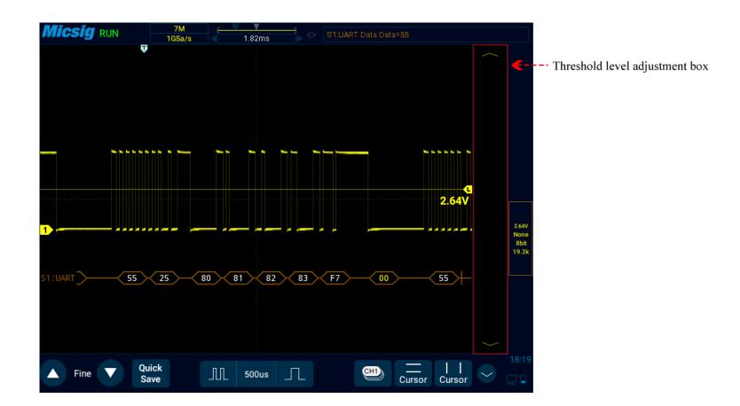
Figure 12-7 UART Decode Level Adjustment
