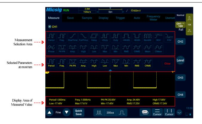
Figure 7-1 Automatic Measurement Menu
