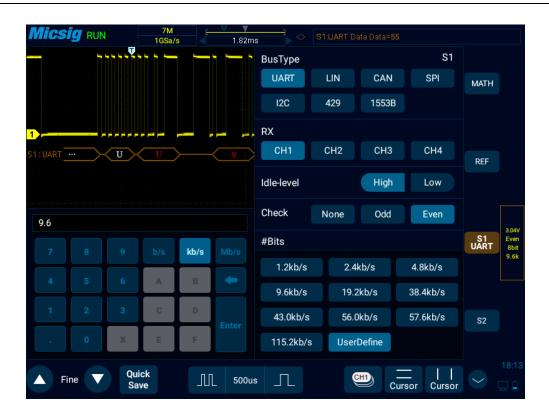
Figure 12-5 Baud Rate Default Setting
