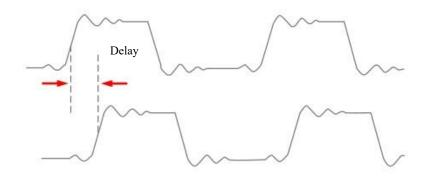
Figure 7-5 Delay Measurement Schematics
