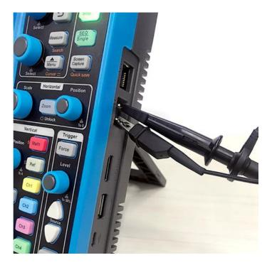
Figure 2-13 Probe Connection
