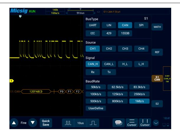
Figure 12-14 CAN Bus Configuration Menu
