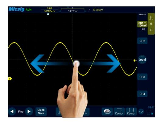
Figure 4-2 Move the Waveform Horizontally on the Screen
