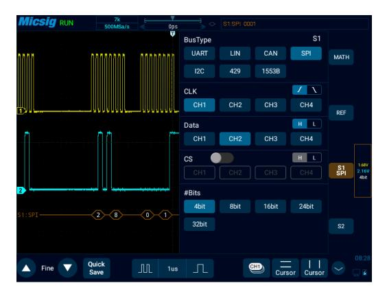
Figure 12-18 SPI Bus Configuration Menu
