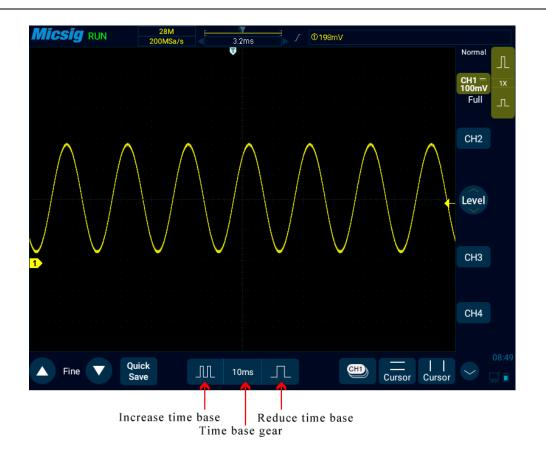
Figure 4-3 Adjust the Horizontal Time Base
