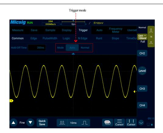
Figure 6-5 Oscilloscope Trigger Mode Setting
