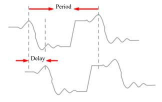
Figure 7-6 Phase Measurement Schematics
