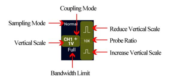
Figure 5-3 Channel Display Interface
