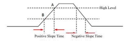
Figure 6-25 Positive/Negative Slope Time
