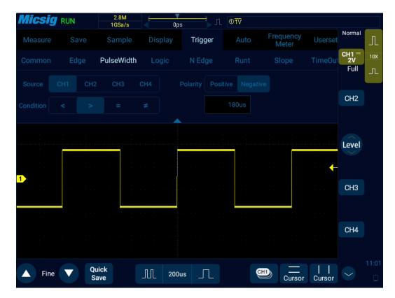
Figure 6-14 Negative Polarity Pulse Level Flip
