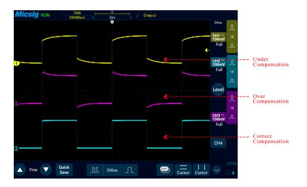
Figure 2-14 Probe Compensation
