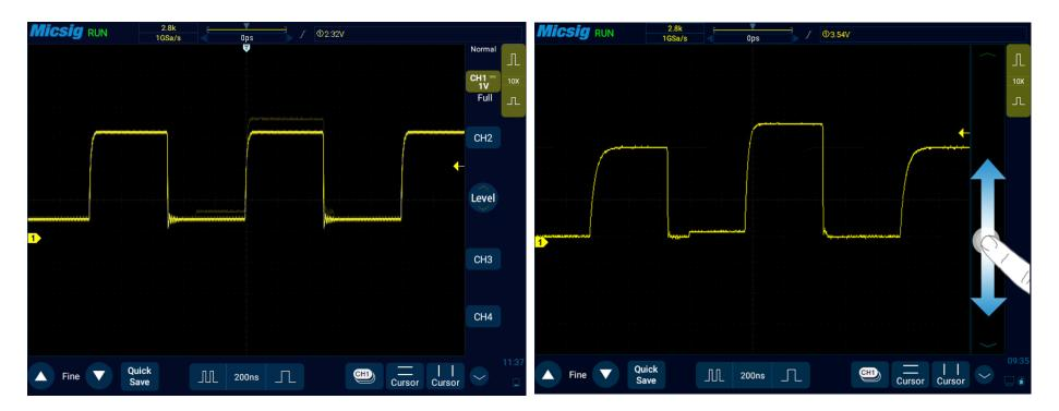
Figure 6-3 Abnormal Signal in Periodic Signals
