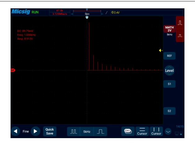
Figure 9-4 Spectrum Amplitude as V-Hz
