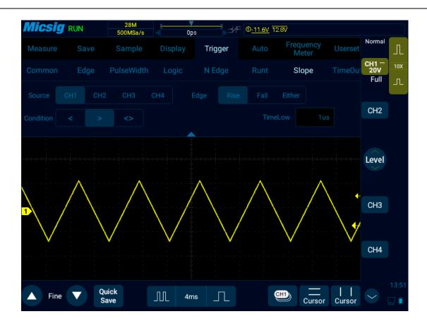
Figure 6-26 Slope Trigger Setting Menu
