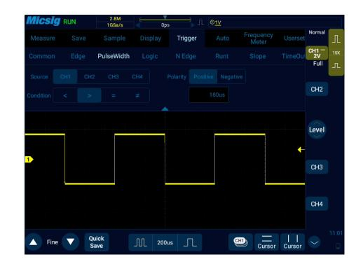
Figure 6-13 Pulse Width Trigger Setting Menu
