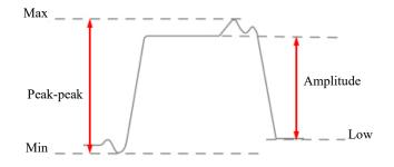
Figure 7-7 Voltage Measurement
