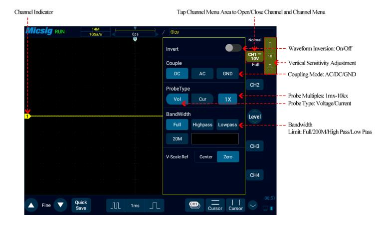
The figure below shows the "CH1 Channel Menu" displayed after opening the CH1 channel menu.
