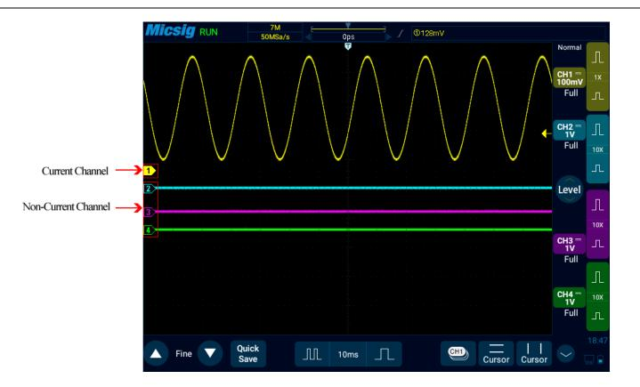
Figure 5-2 Current Channel and Non-Current Channel
