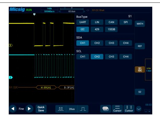
Figure 12-22 I2C Bus Configuration Menu
