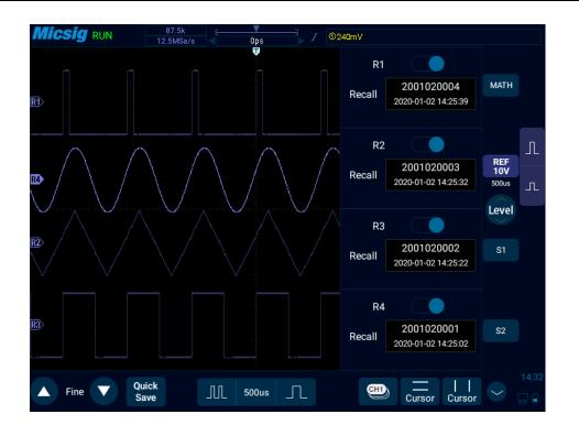
Figure 9-6 Restore Reference Waveform
