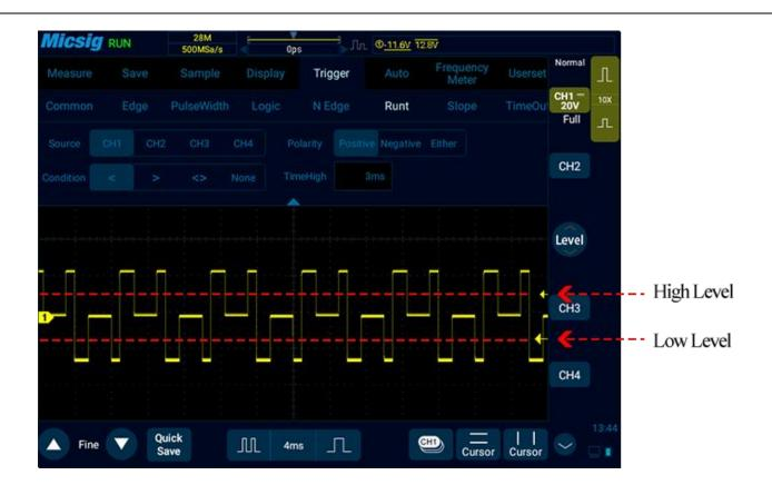
Figure 6-24 Runt Trigger Setting Menu
