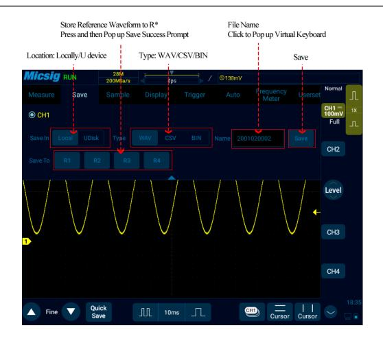
Figure 8-4 Save CH1 Reference Waveform Interface
