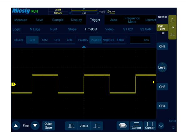
Figure 6-28 Time-out Trigger
