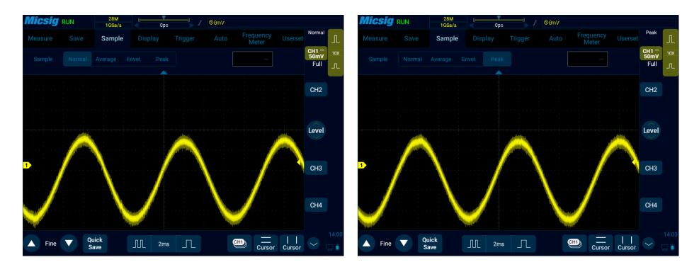
Figure 11-5 Sine Wave with Burr
