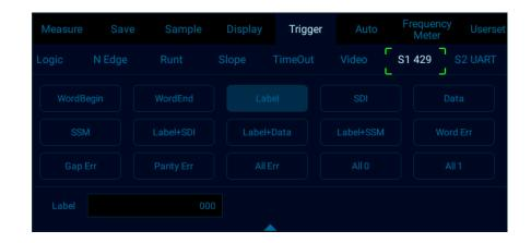
Figure 12-27 ARINC429 Trigger Mode Configuration Menu
