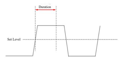
Figure 6-27 Timeout Trigger Schematics
