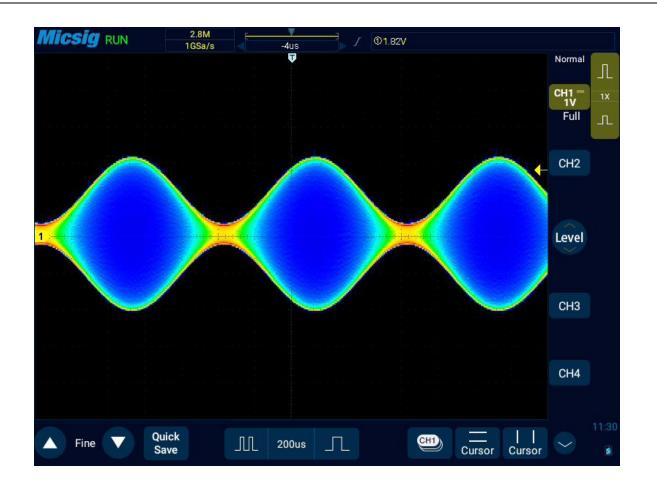
Figure 10-5 Color Temperature Open Mode
