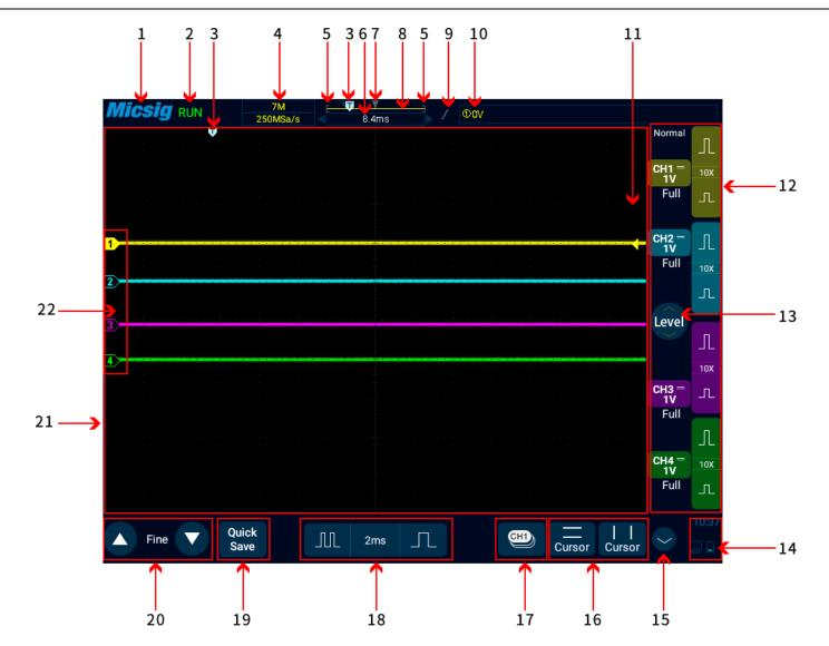
Figure 2-5 Oscilloscope Interface Display
