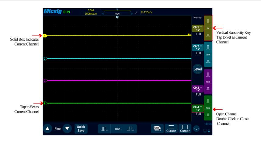
Figure 5-4 Channel Open, Close and Switching
