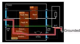
To perform tests safely, it is necessary to check in advance that the measurement point is not grounded.
