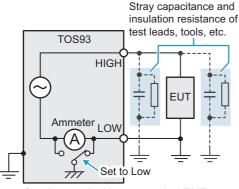
Can be used with a grounded EUT
