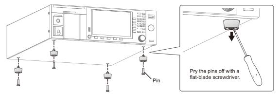
Pry off the pins holding the legs (four locations) with a flat-blade screwdriver.
