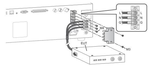
**3** Connect the insulation transformer to the AC LINE IN inlet with the power cord for the EUT.
