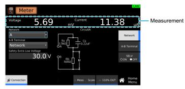
If Measuring across terminals A and B (A-B Terminal) (p.173) is set to VoltMeter and voltage exceeding the value set with SELV setting (p.174) is present across terminals A and B, the DANGER LED lights.
