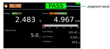
When a test finishes, the judgment result is shown in the test status.
