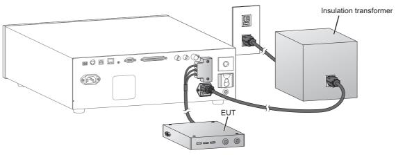
After the test leads are connected
