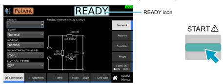
"TEST" is shown in the upper right of the display, and the test starts. If the test does not start, see "Unable to start a test" (*p.288*).
