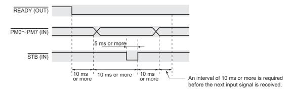
With "READY" shown in the upper right of the display, apply high-level or low-level signals to PM0 (pin 3) to PM7 (pin 10) of the SIGNAL I/O connector.
