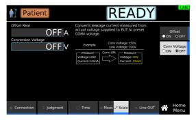
**3** If you select on, use the numeric keypad or the rotary knob to enter the voltage. Setting range: 80.0 V to 300.0 V This completes the setting.
