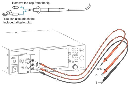
The locations on the EUT that test leads are connected to vary depending on the probe and condition settings of the test conditions and the appliance class of the EUT. For details on touch current testing, see "Connecting the test leads to the EUT" (p.120). For details on patient leakage current testing, see "Connecting the test leads to the EUT" (p.162).
